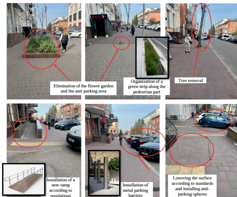
Fig. 2. Problem areas on the pedestrian part of the fragment of Gogol Street in Poltava (Ukraine) and proposals for their solution. Author – Natalia Novoselchuk [from N. Novoselchuk scheme]
