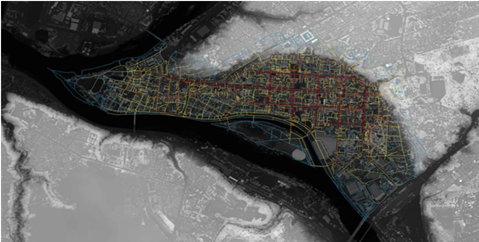
Fig. 3. Segment graph: Integration with a radius of 800 meters. Red colour shows high, blue – low numerical values
