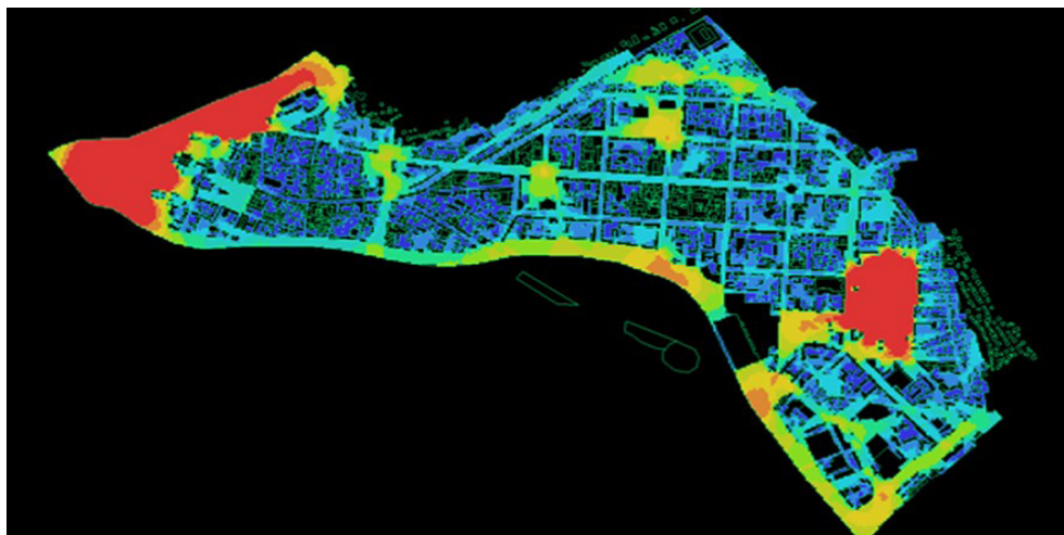
Fig. 4. Visual graph: Connectivity within radius 200. Red colour shows high, blue – low numerical values
