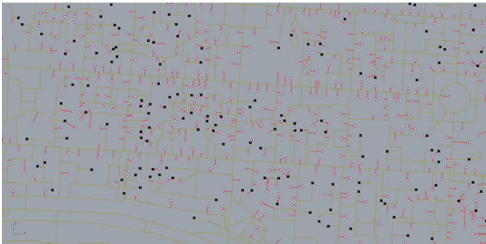
Fig. 5. Part of the building graph of the investigated area in Kaunas created while using the Urban Network Analysis Toolbox (UNAT) [16]. Yellow lines represent segments of streets, white round dots - buildings as graph nodes, red lines - connections between buildings and streets, and black crosses - dead ends of street segments
