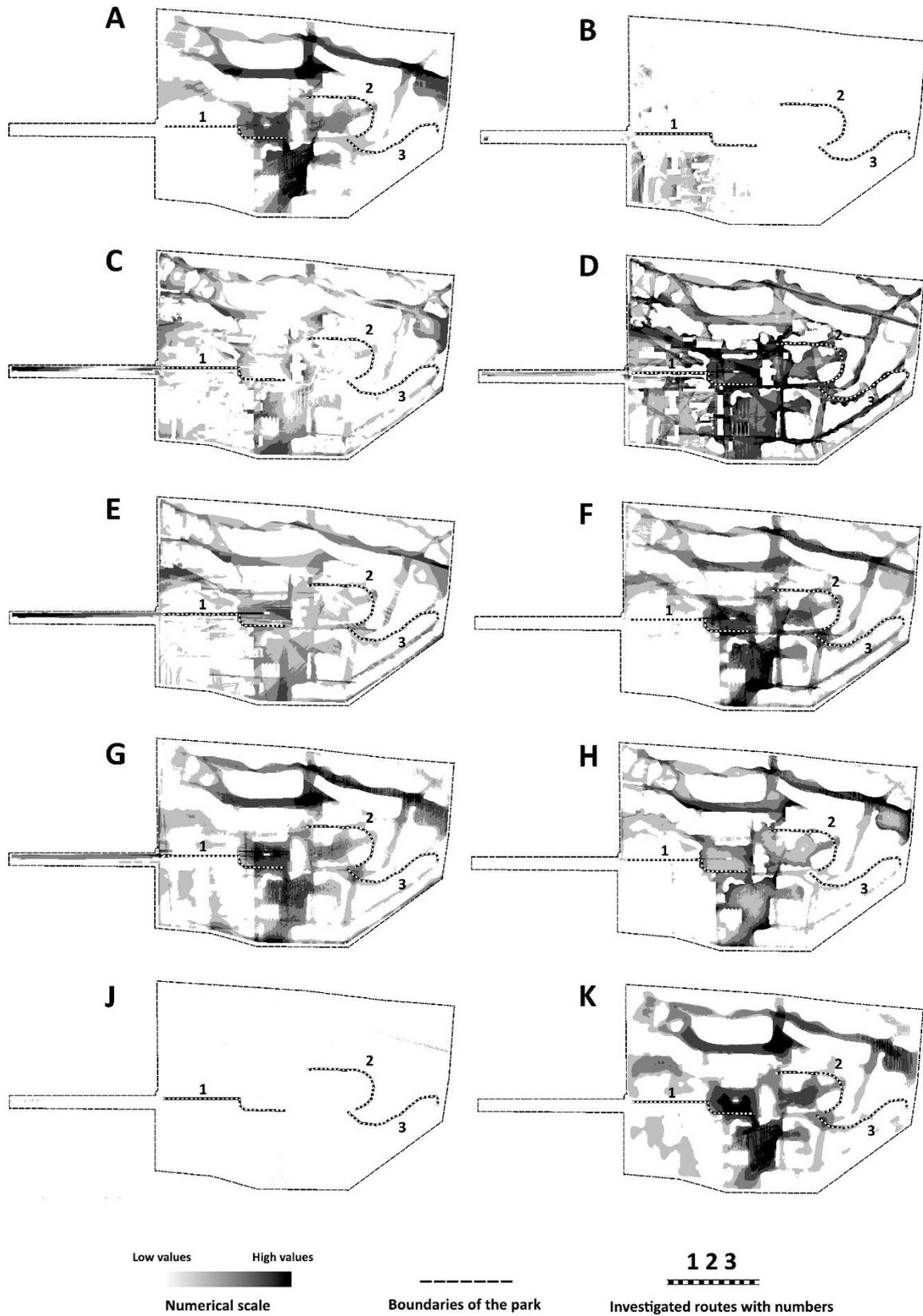
Fig. 3. Properties of the isovists: A – area, B – compactness, C – drift, D – occlusivity, E – vista length, F – perimeter, G – closed perimeter, H – variance, J – skeness, K – average radius
