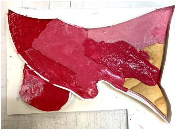
Fig. 5. Plywood geometries are being almost totally covered with a liquid rubber molding agent. Pigment is just added before stirring it up so that it could be seen if the rubber mix has become uniform with the catalyzer.
