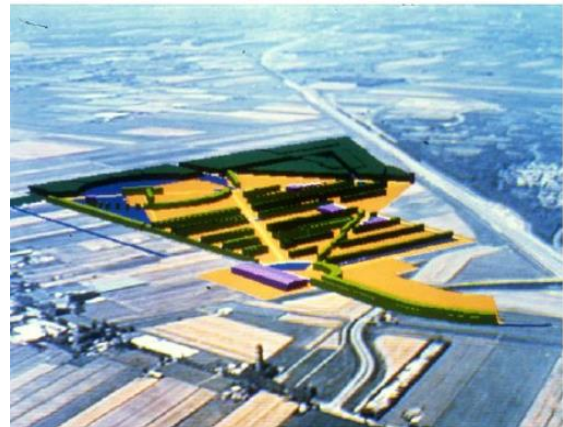
Fig. 3. An early experiment with CAD and 3D modeling: the design for the 1992 Floride in Zoetermeer, Netherlands is constructed in three dimensions in a digital environment and draped on aerial photograph of existing situation [20]
