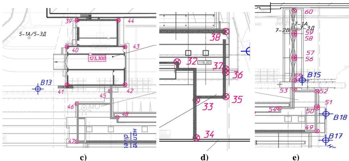
**Figure 3.** Installation scheme of control marks on the Northern (a) and Southern (b) basements of the NSC Service Zone, settlement deformation marks on the southwestern end wall (c) Arches of the NSC (marks 39 – 48), settlement deformation marks on the north-eastern (d) (marks 32 – 38) and south-eastern (e) (marks 49 – 60) end walls of the Arch of the NSC
