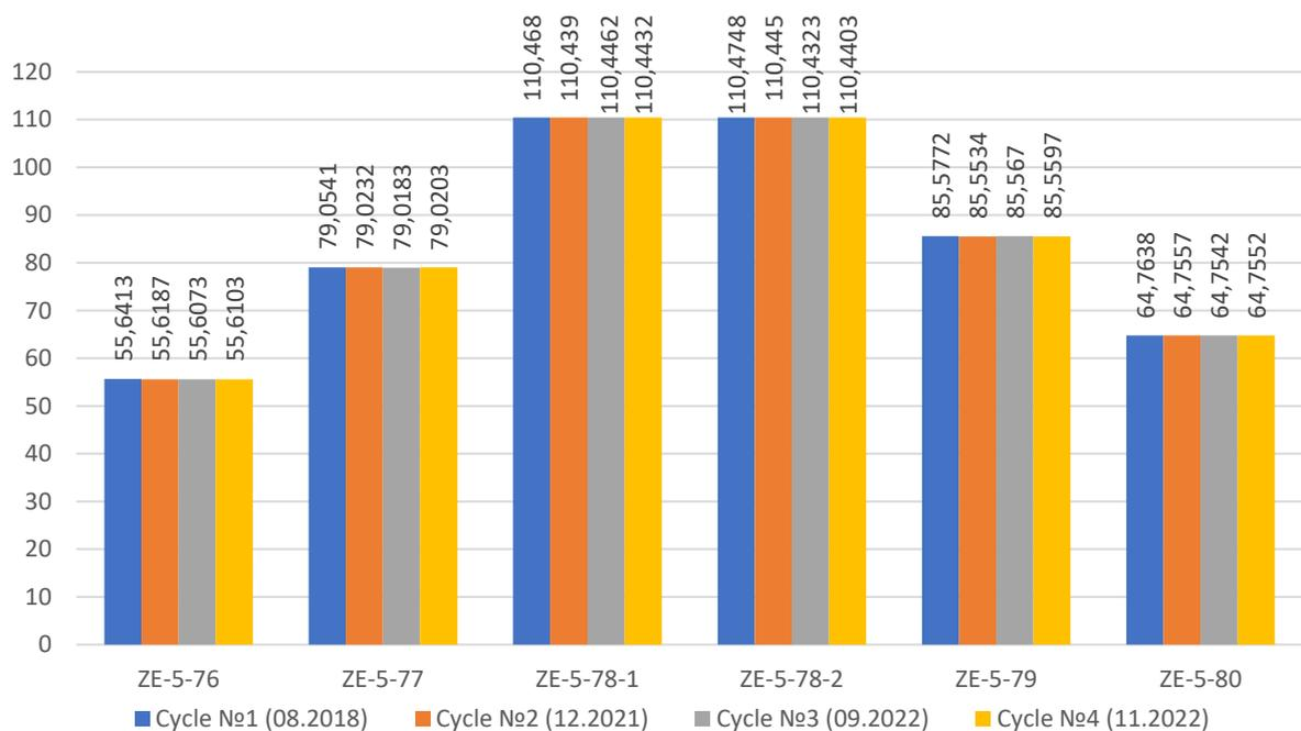
**Figure 4.** Vertical displacements for four cycles of measuring control marks of the NSC Arch structures, m
