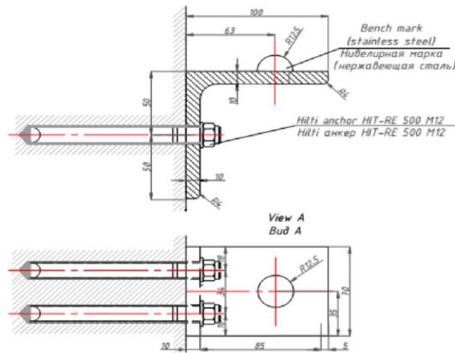
**Figure 2.** The construction of a settling deformation mark
